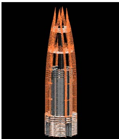
Figure 6. Finite Element Analysis Model of Spire and Crown
